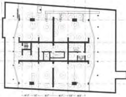
Fig. 4 above Basement plan of tower block
