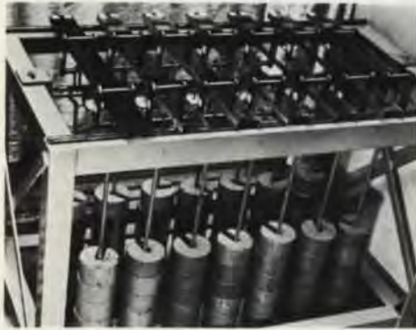
Fig. 17 Laminated glass beams under sustained loading
