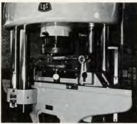
Fig. 19 Arrangement for fatigue loading of laminated glass test beams
