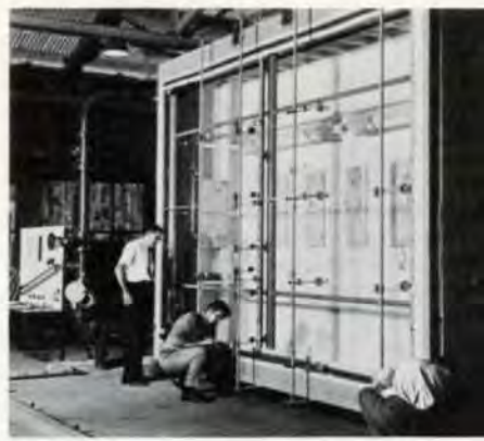
Fig. 20 Full-scale loading of laminated glass plates
