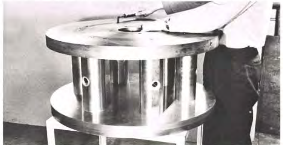
Fig. 6 Assembly of 6000 kN pile load cell
