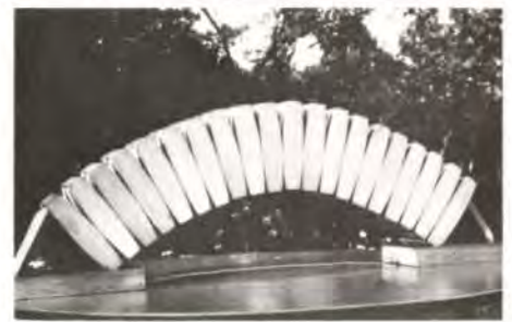
Fig. 1 Model of arch formed of radiused voussoirs which allow the line of thrust to move in response to point loads. This model was made by Frei Otto to demonstrate the principle of inverting a hanging chain
