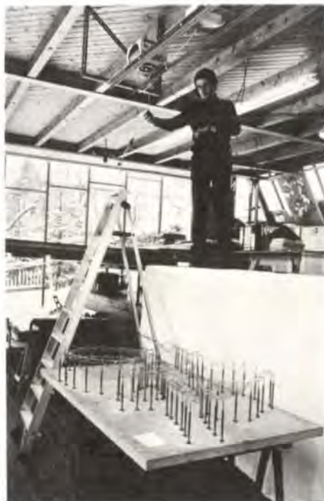
Fig. 13 Stereo photography of hanging chain model by IAGB
