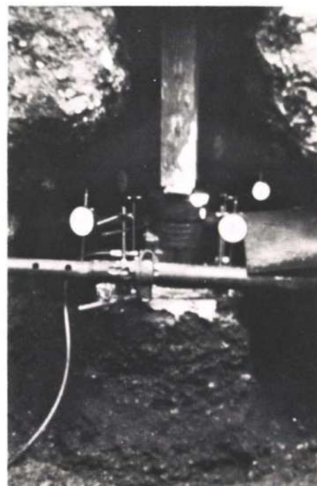
Fig. 4 right Plate loading test on unconfined cube of gravel cut from chemical grout treated zone (Photo: Michael Courtney)
