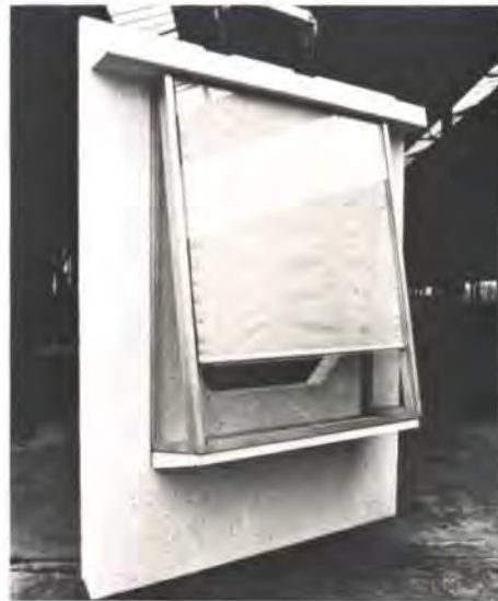
Fig. 41 'Window' with sunblind half down. Ventilation occurs behind the plane of the blind
