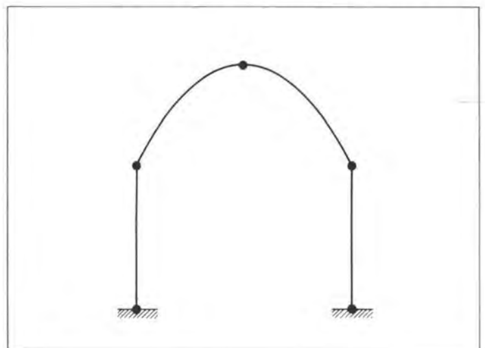
Fig. 1c Collapse of a portal frame
