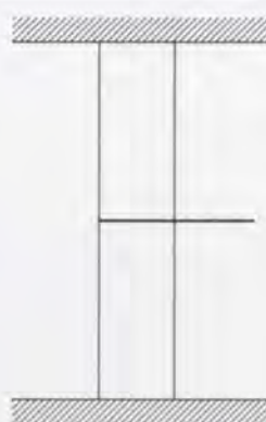
3. Both hangers prestressed.
