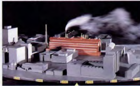
△ 10. Wind tunnel tests for fume dispersal.
