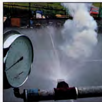
3. Discharge pattern of long throw head.
