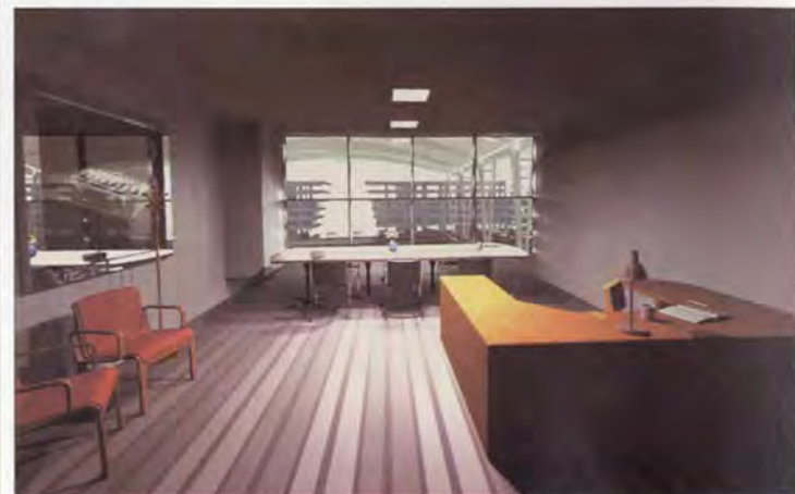
4. Daylight penetration into interior of office, generated by the RADIANCE light visualization program.
