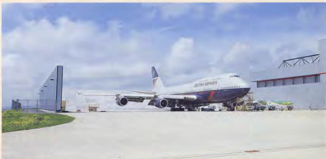
A. Aircraft City of Norwich in acoustic ground run enclosure.
