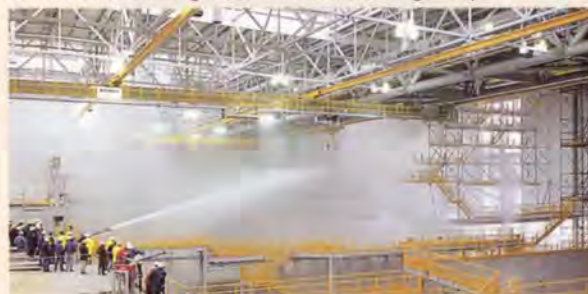
B. Full scale discharge test in the double hangar bay.
