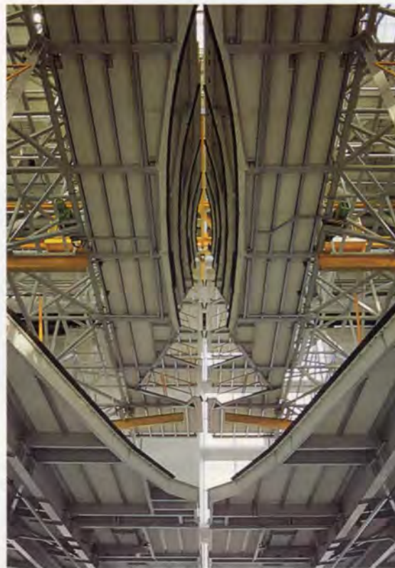
◀ A. Tail docking view from hangar floor showing platform profiling.
