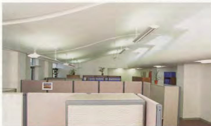
9. Office with high curved ceiling and high level roof vents which dissipate hot air trapped above occupied zone.
