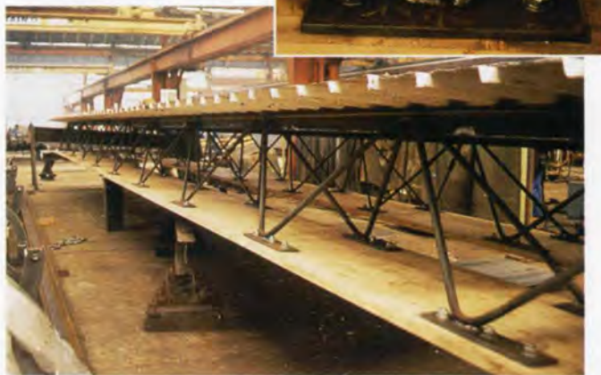
24. Prototype trusses ready for load testing.
