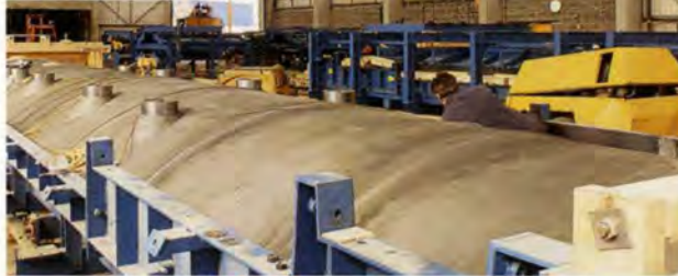
9. Steel moulds for floor units.
