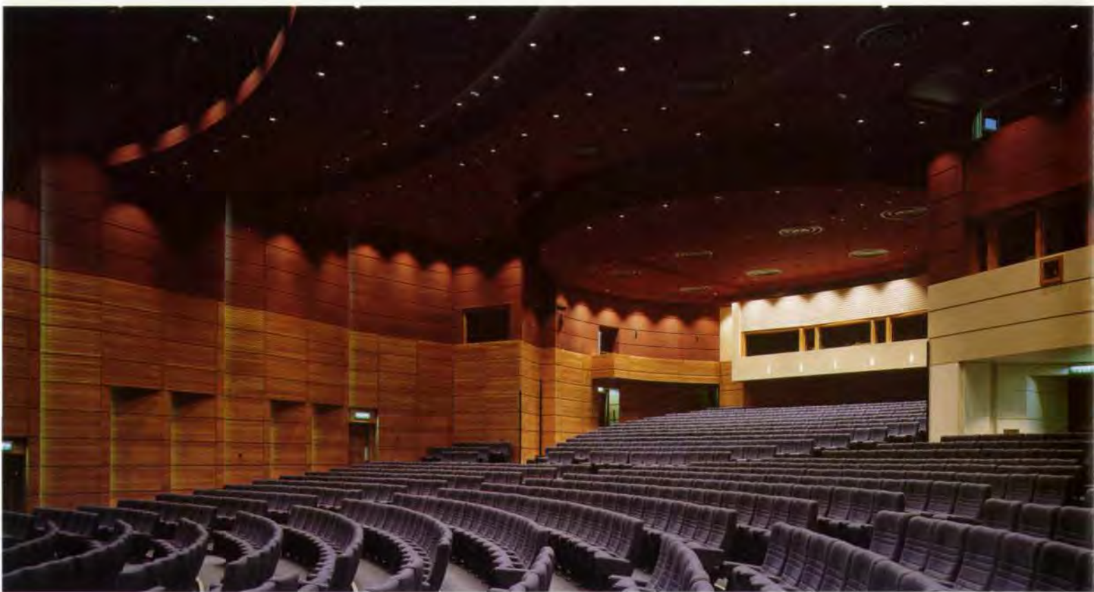
15. The auditorium with one rotatable section facing forward; the main lighting is by recessed, dimmable downlighters.
