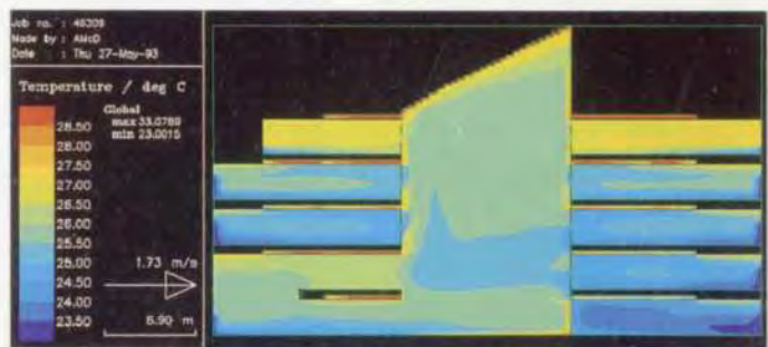
Above 6. CFD analysis using AIRFLO 3D. Below 7. Environmental control strategy.
