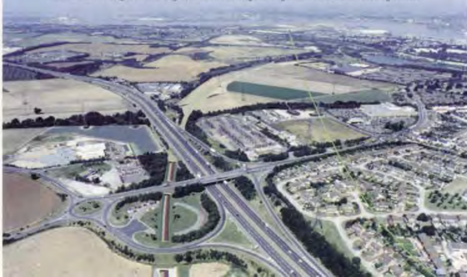
1. Pepper Hill: This superimposition shows the final route (left) in a cut-and-cover tunnel under the A2/B2175 intersection. The green line (right) shows the original alignment under the housing estate.
