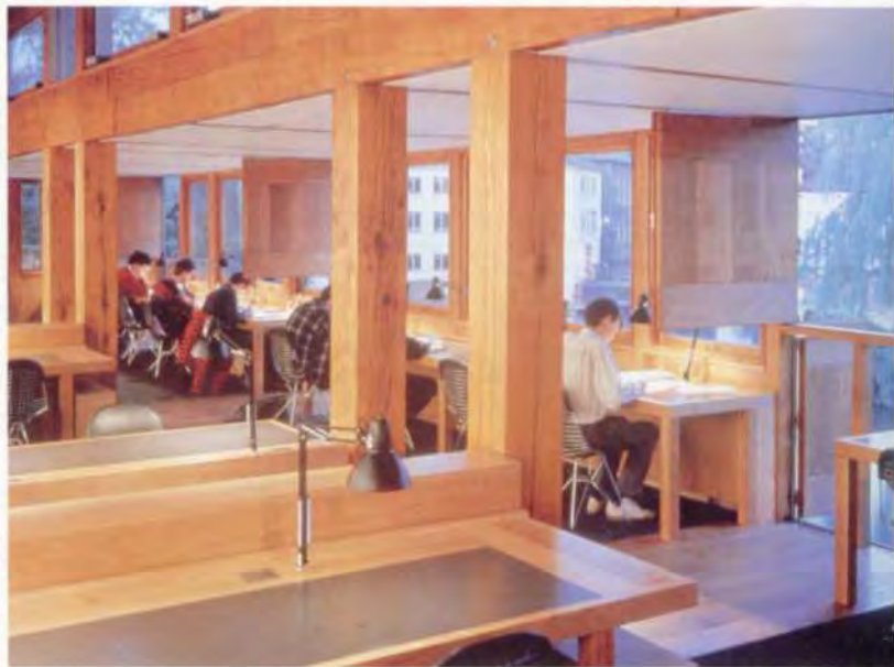
5. The study area, showing oak timber structure and 'stable' doors giving natural ventilation.
