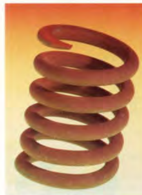
8. Macro defect-free cement (MDF) spring; such a structure, a few centimetres long, is only achievable due to MDF's high tensile and compressive strength.
