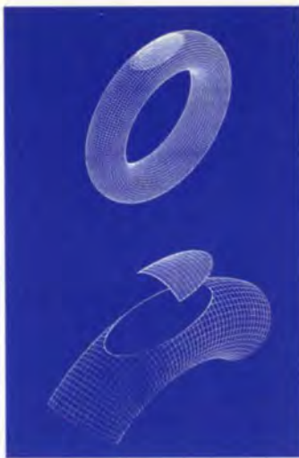
4. Definition of the torus geometry to accommodate the B52 plane: major radius 277m, minor radius 63m.
