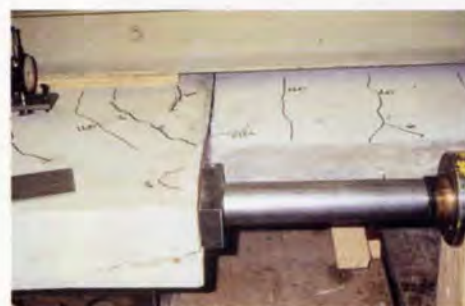
14. Laboratory tension tests on 100mm roof panels.
