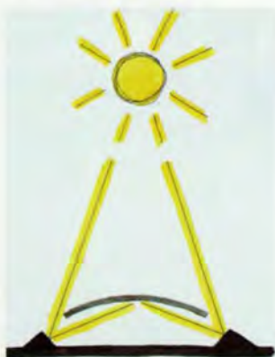
19. Pathway of natural light through perimeter lighting slot.
