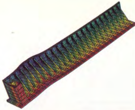
4. NASTRAN FE analysis of the quay wall.
