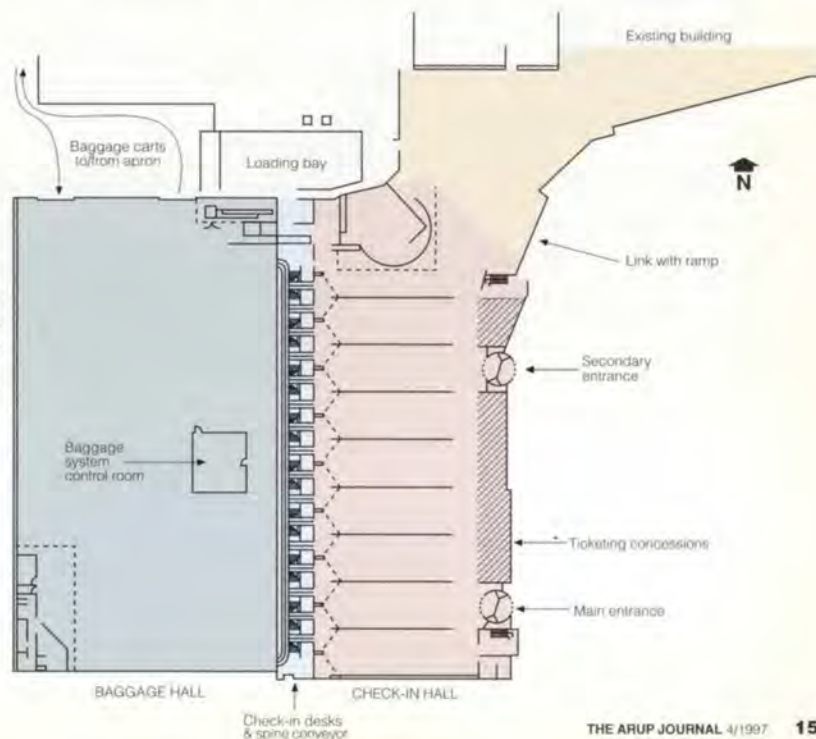
5. Plan showing the two main parts of the Departure Building: The baggage hall and check-in hall.
