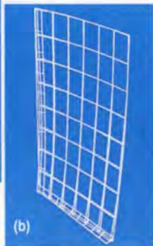
(b) when subjected to blast loading it begins to deflect...
