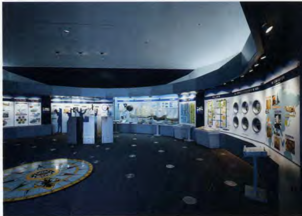
12. The core structures contain exhibition areas; note air-supply grilles on the floor.
