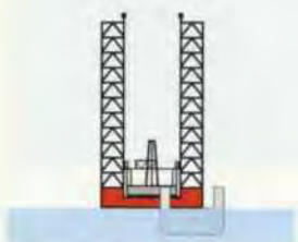
Offload and wet tow to offshore field (can be towed if more economic).
