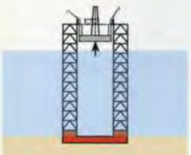
Raise deck, weld deck to legs, remove strands, commission.
