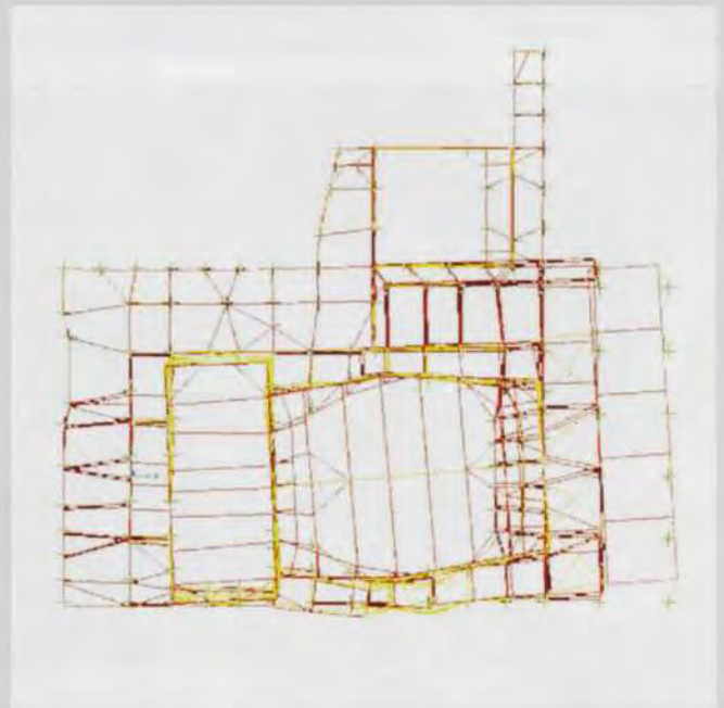
8. Plan view - Mode 3 deflected shape with mass accelerating transversely with torsion.
