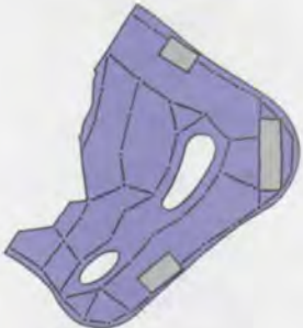
Framing option 2: Irregular column grid.
