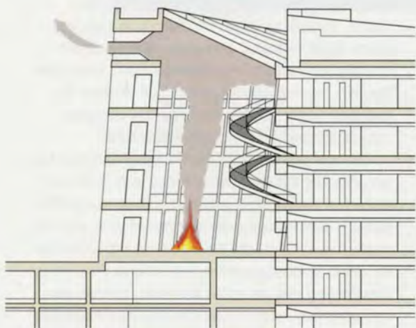
10. Smoke extract strategies for the atria saved costs significantly.
