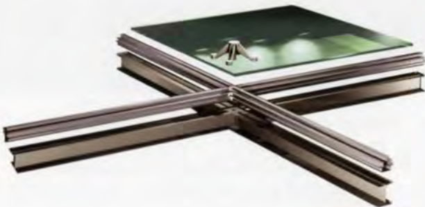
5. Detail of Federation Court roof 'spider' clamp.
