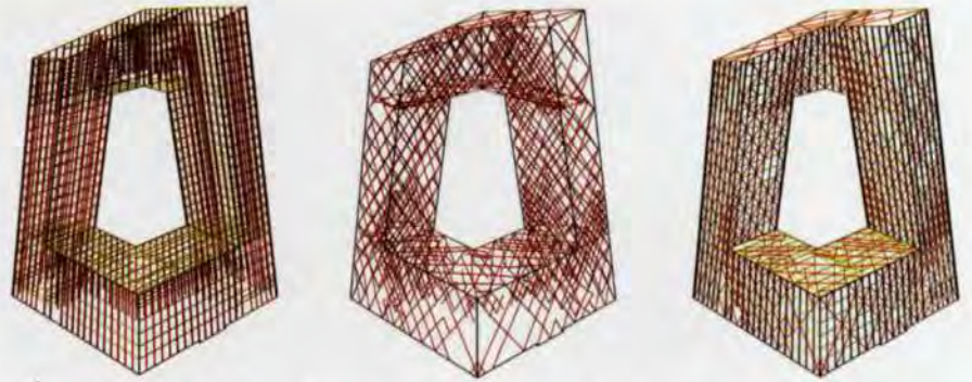
4. Principles of the tube structure: regular grid of columns and edge beams + patterned diagonal bracing = braced tube system.
