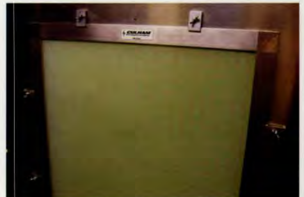
2. A 5.2GHz bandstop FSS.
