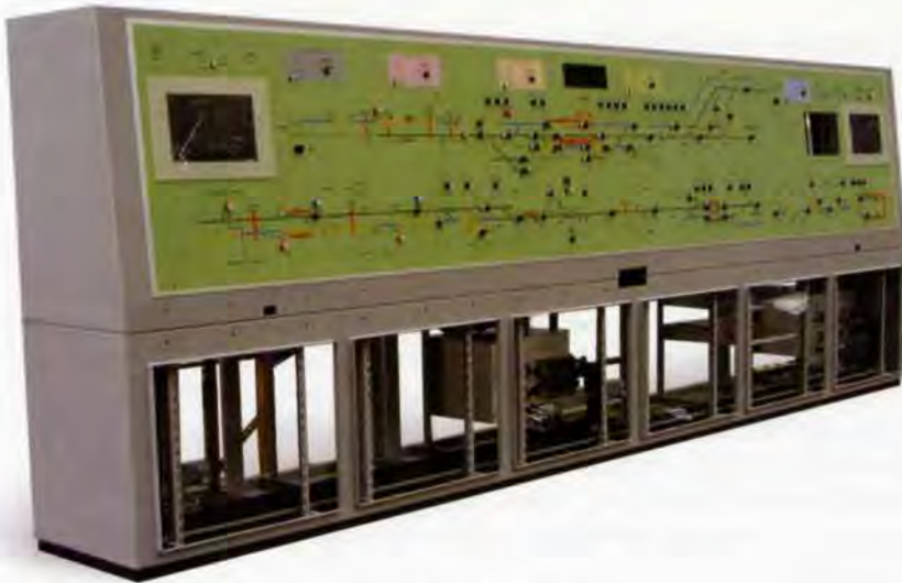
3. Signalman's panel being manufactured in the GE factory.
