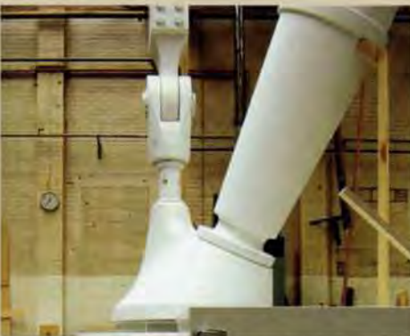
d) Casting manufacturer's half-scale prototype.
