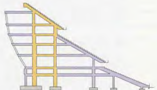
10. Corner section; the part of the structure that contributes most to stability is highlighted.
