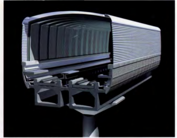
12. Design for full noise enclosure at crossings.
