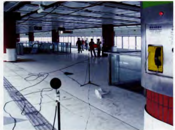
6. Acoustic RT testing at Kam Sheung Road station.
