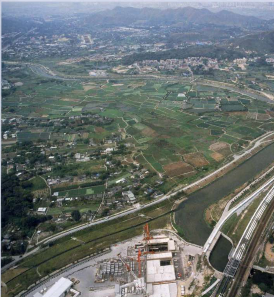
2. Aerial view of Long Valley during construction of the Lok Ma Chau spur line. At the foot is the TBM launch shaft at Sheung Shui; in the distance, the excavation for the Kwu Tung station enabling works.
