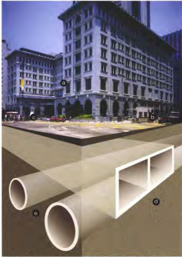
3. Nathan Road crossing, envisaged as an in situ box to accommodate a possible integrated basement car park for the hotel: (a) Peninsula Hotel, (b) Nathan Road, (c) Salisbury Road, (d) KSL tunnels, (e) MTR Tsuen Wan line.
