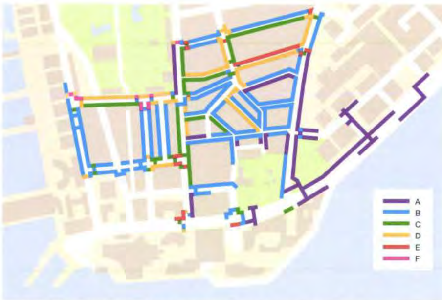
5. Levels of service at pedestrian links: "A" represents the least busy, and "F" is "congested".
