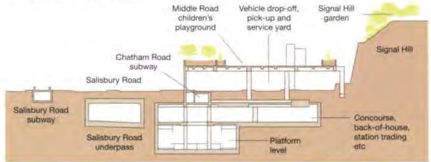
a) Section through the west end, beneath the Middle Road children's playground.
