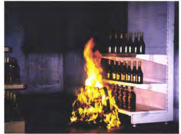
6. Cabin concept full-scale fire test.
