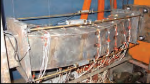
10. Twisted thin-walled box secondary member being tested at Beijing Tsing Hua University.
