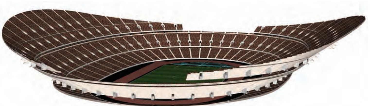
4. Like most modern stadia, the “Bird’s Nest” was designed inside out, beginning with the bowl.
