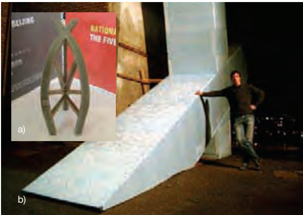
15. (a) Small-scale card prototype; (b) Full-scale foam board prototype.
