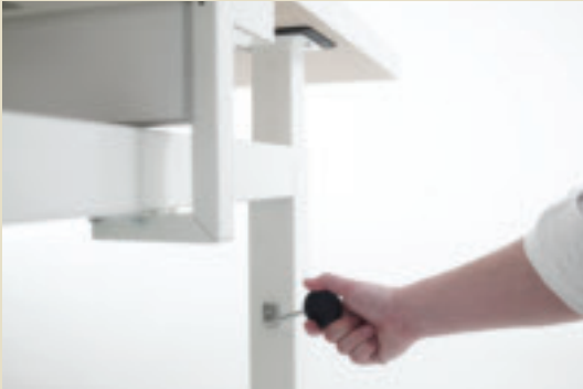
3. Height adjustment is achieved using an Allen key. The level can be read on the inscribed scale on the back of the leg.
