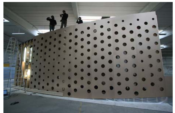
10. March 2009: Timber mock-up to test the scale, perforation principle, and lighting devices.
