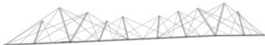
As-built masts and cables on the upstream side, with geometry refined by small random offsets to tops of masts.
