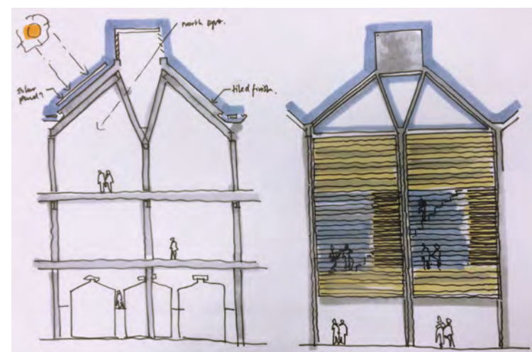
10: The pitched roofs help to manage high levels of seasonal rainfall
