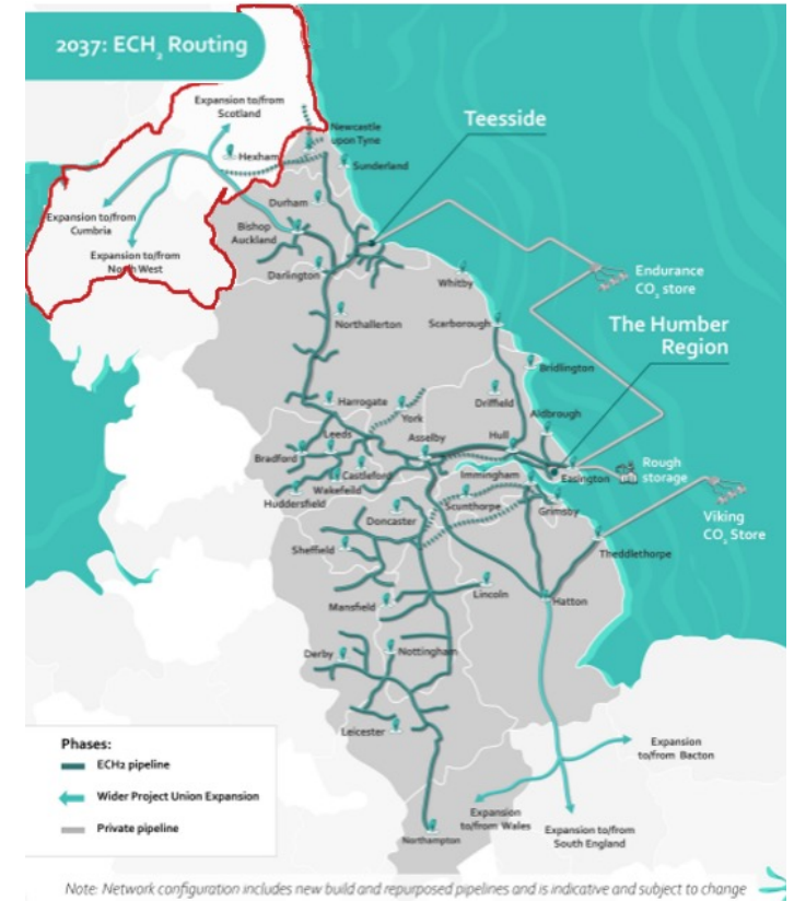
Figure A1: System boundary of storage demand modelling assessment, chosen to align with East Coast Hydrogen Delivery Plan system boundary with additional to include full Northern LDZ region (as outlined in red). [12][13]
