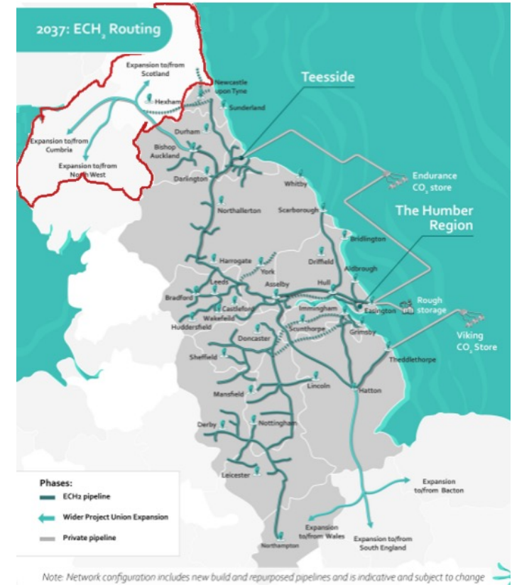
Figure 6: System boundary of storage demand modelling assessment, chosen to align with East Coast Hydrogen Delivery Plan system boundary with additionality to include full Northern LDZ region (as outlined in red). [12][13]
