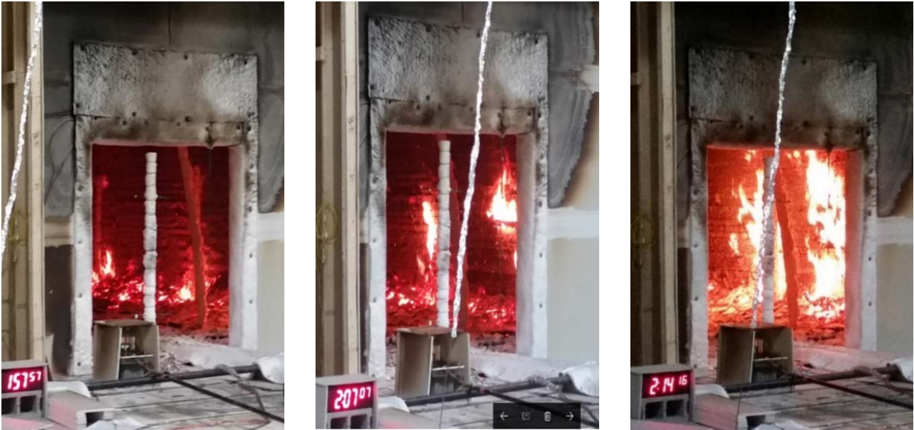
Figure 17: CLT compartment fire experiment with timestamps showing an example of secondary regrowth (Su et al., 2018b).
