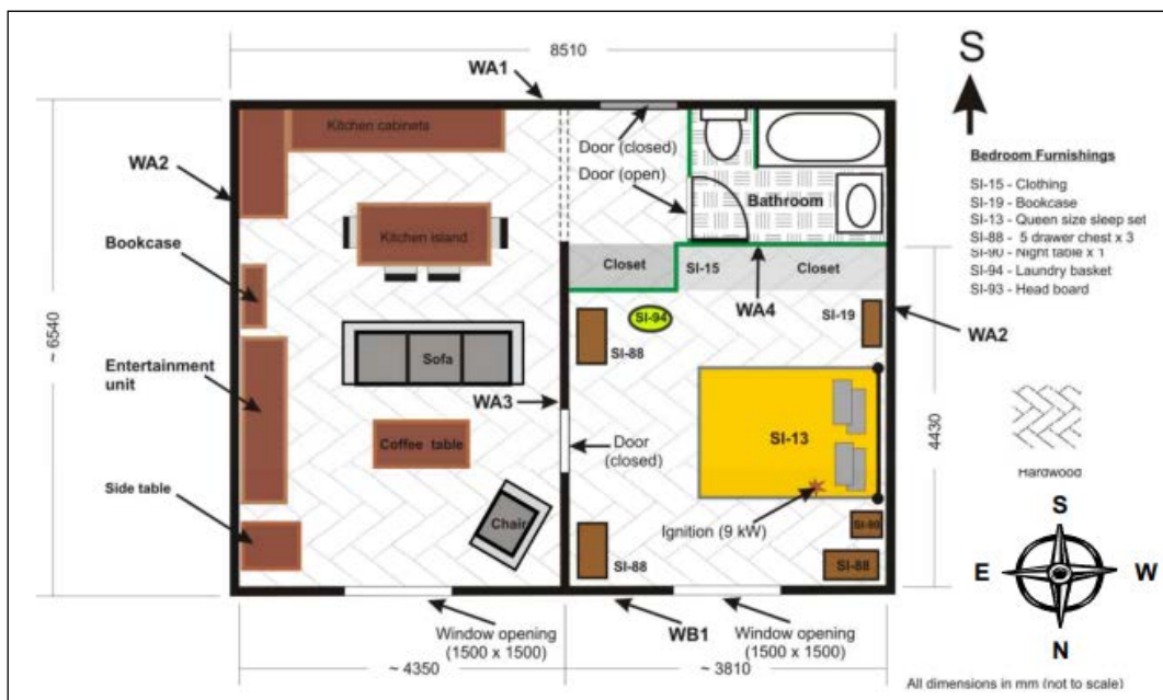
Figure 21: Layout and residential fuel load in the experiments of Su and Lougheed, 2014.
