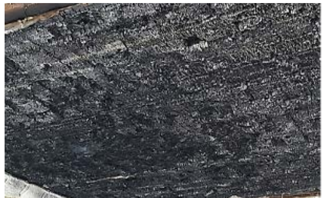
CLT panel post test with bond line integrity in fire.
