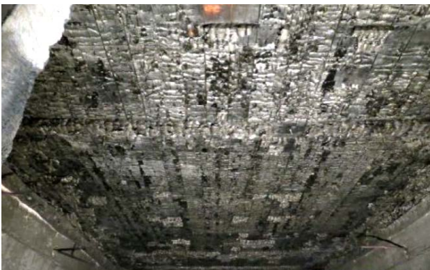
CLT panel post fire test without bond line integrity in fire.
