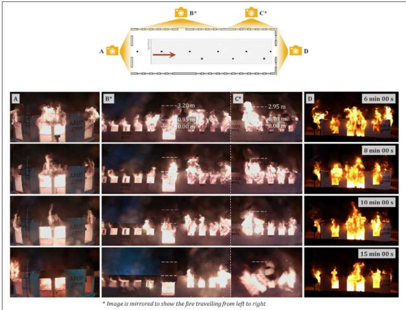
Figure 76: External flaming from various openings during the CodeRed #01 experiment.
