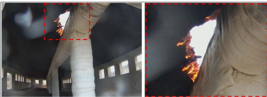
Figure 74: Transition to flaming observed at a smouldering hole 37.5 h after the end of flames in CodeRed #01
