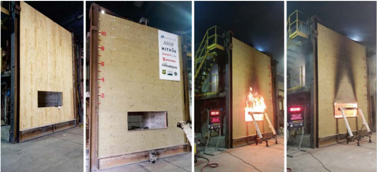
Figure 80: Timber wall subjected to an NFPA 285 test. Left to right: exposed; encapsulated with mineral wool and gypsum board; during fire test; after fire test (Barber and Blomgren, 2023).
