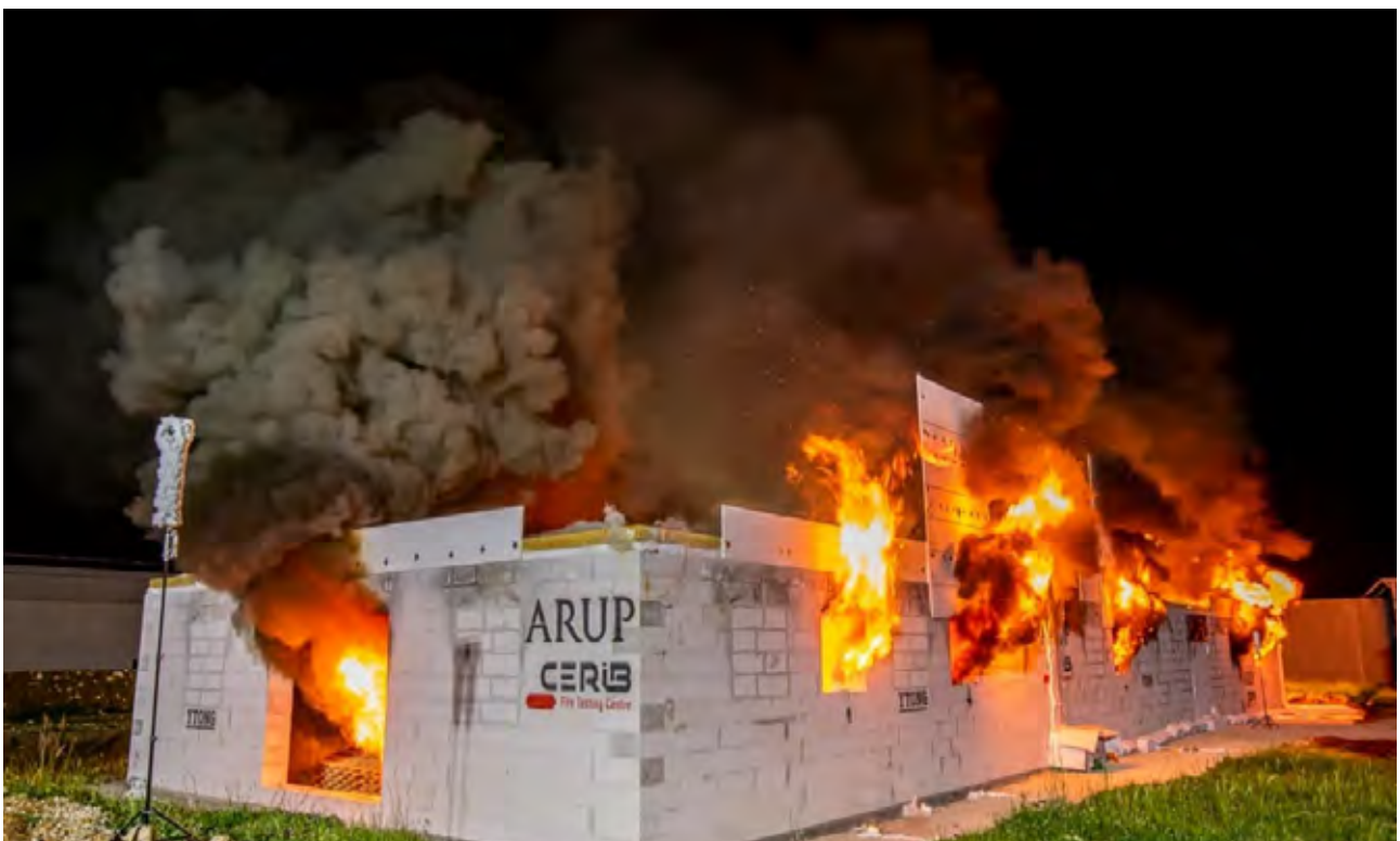
Figure 4. Photo from experiment two showing extensive external flaming from openings, as the fire reaches the end of the compartment. Wooden crib at the end of the compartment has not yet fully ignited.
