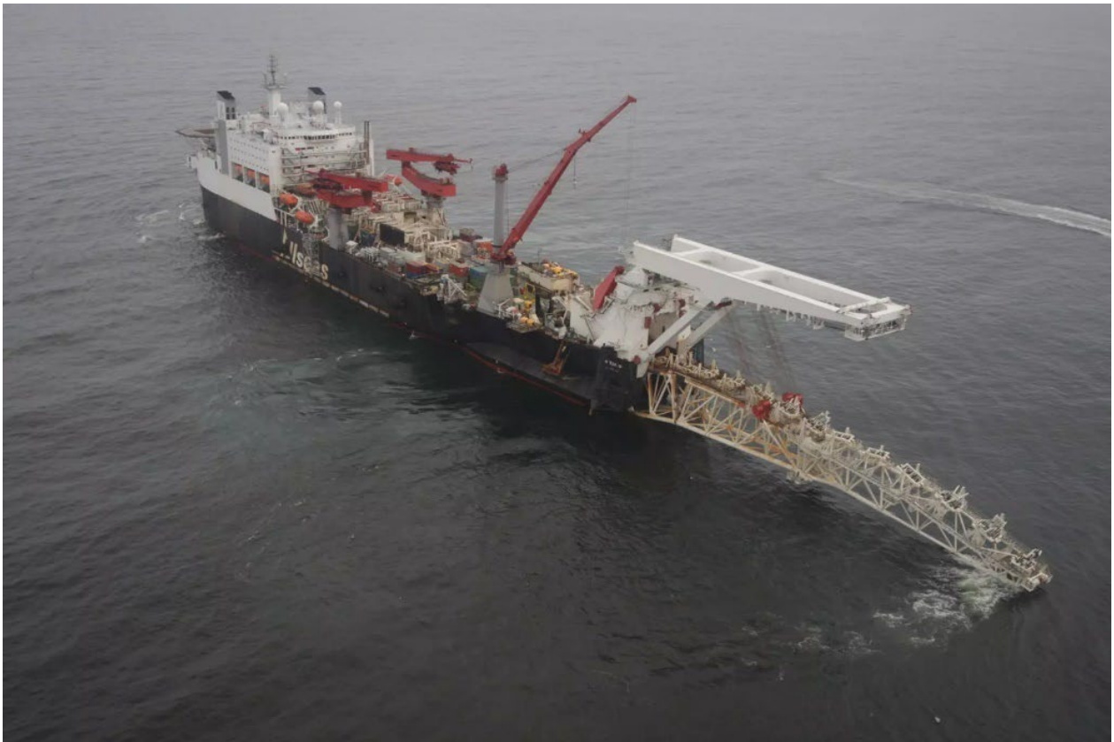
Figure 65: Typical S-Lay Vessel – Allseas Solitaire (© Allseas)
