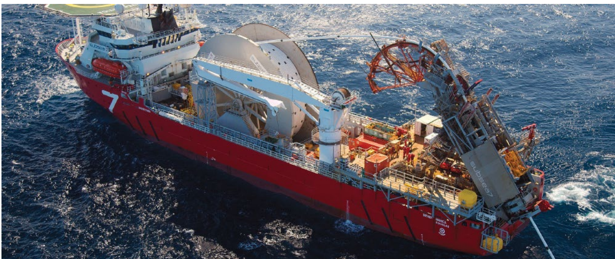
Figure 68: Typical Reel Lay Vessel – Subsea 7 Seven Navica (© Subsea 7)
