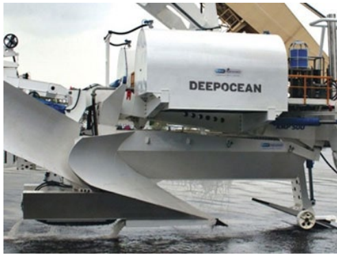
Trenching Plough © Delta Subsea Deepocean
