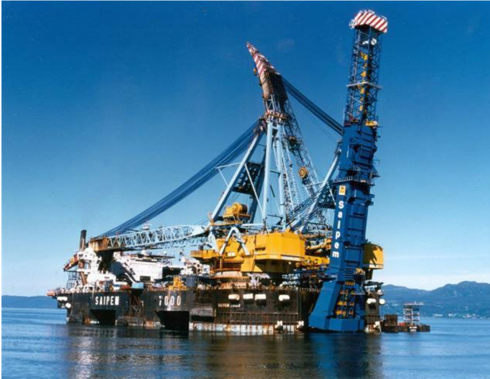
Figure 67: Typical J-Lay Vessel – Saipem 7000 (© Saipem)
