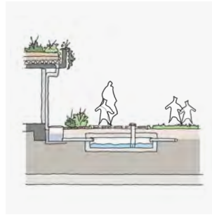
B.4 Below ground attenuation tank
