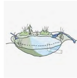
A.5 Detention basin
