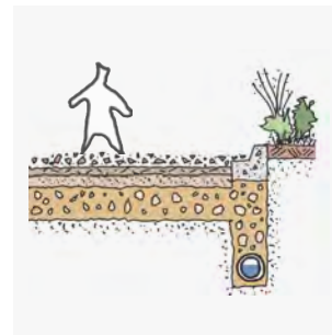
A.9 Permeable surface: woodchip
