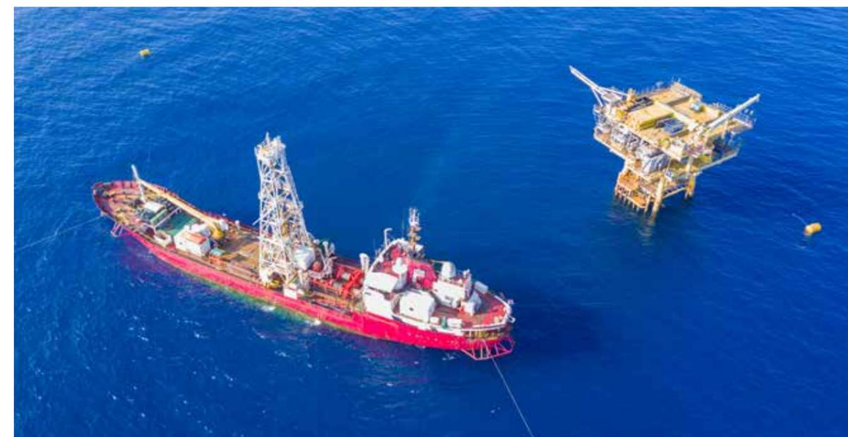
**Figure 7** Offshore geotechnical drilling vessel
