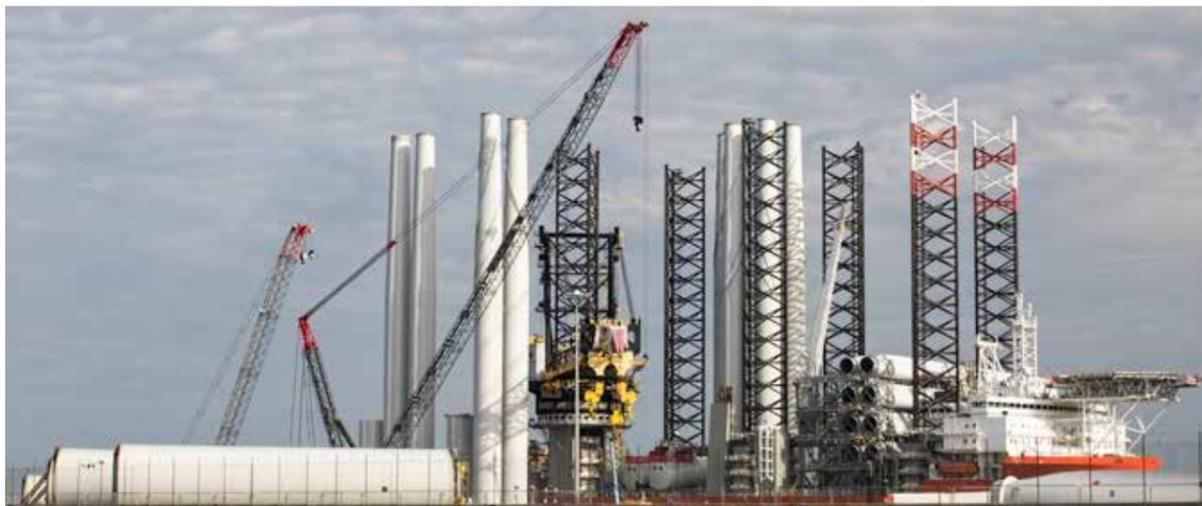
**Figure 22** Self-propelled jack up vessel in port Great Yarmouth, UK
